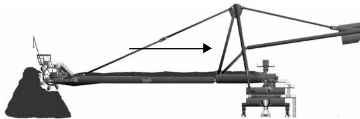
Masted boom configuration length over 38 m
